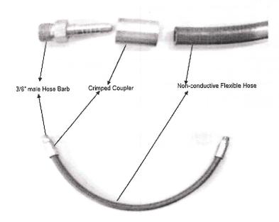
fabricated flexible hose must be suitably fitted to 3/8\*BSP\*3/8 push fit connector.
